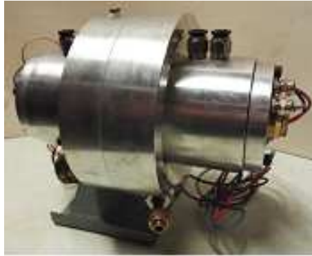
Figure 5: View of microturbine in RC application.
