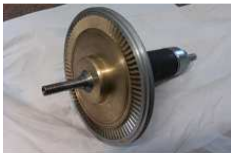
Figure 4: Turbine rotor disk with generator rotor.
