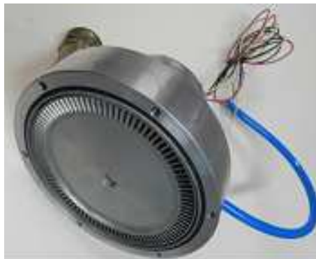
Figure 6: Nozzle disc of microturbine 1st stage.
