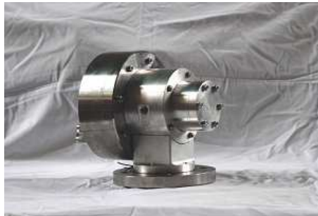
Figure 3: View of vapour ORC microturbine.
