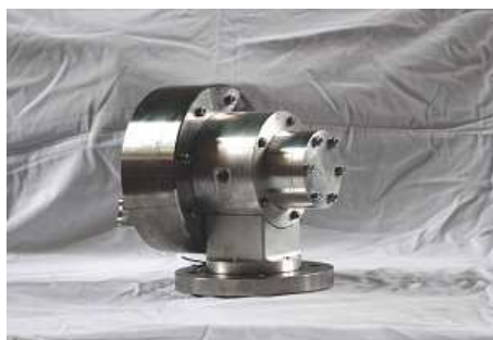
Figure 3: View of vapour ORC microturbine.
