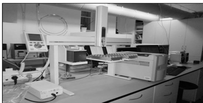
Figure 2. Electronic nose of Fast Gas Chromatography (Fast GC-type)—HERACLES II.
