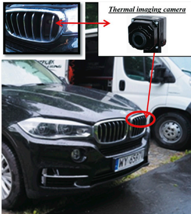
Fig. 10. Arrangement of the infrared camera in the vehicle (by: Grzegorz Motrycz)
