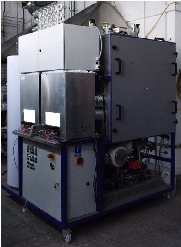
Fig. 30 – Micro-combined heat and power unit with SOFC, design and constructed in the Institute of Power Engineering.
