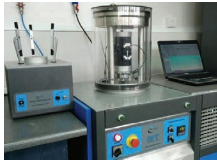
Fig. 3. View of the AMPT/SPT apparatus.
