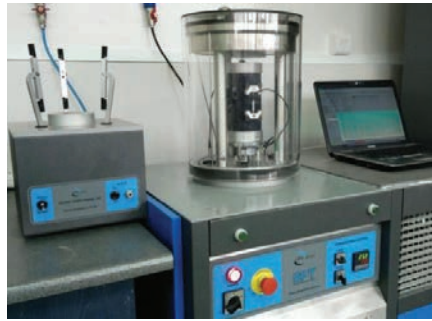
Fig. 3. View of the AMPT/SPT apparatus.
