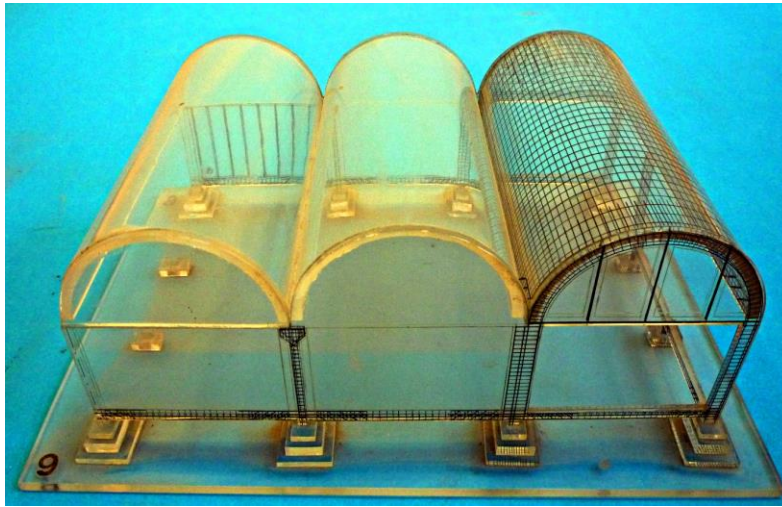
Figure 9: Cylindrical shells with the reinforcement of the shells and columns visible
