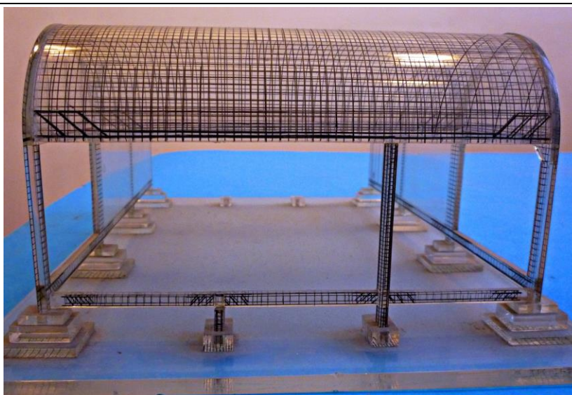
Figure 8: The model of a single-storey, single-aisle reinforced concrete hall covered with three cylindrical shells
