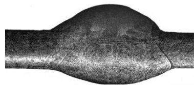
Rys. 5. Złącze spawane Incoloy 800HT/316L, pow. x5 Fig. 5. A cross section for dissimilar welding Incoloy 800HT/316L joint, mag. x5
