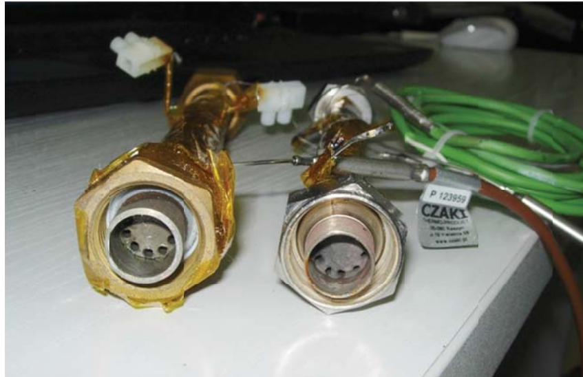
Fig. 3. Evaporators with porous wick materials: Ni-Cu (left) and Ni-Al (right)
