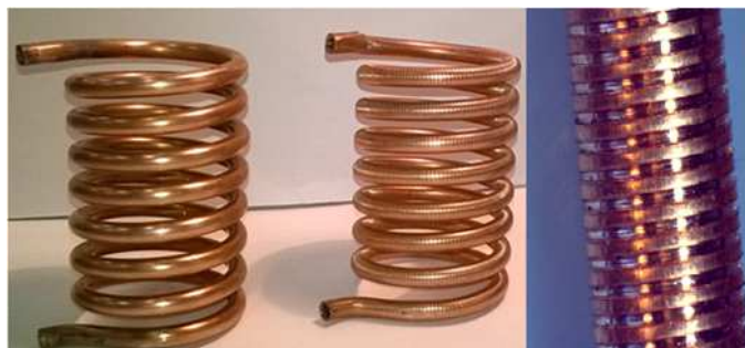
Figure 3: Obtained construction of helical coils: at the left side – coil made from smooth copper pipe, in the middle – coil with modified surface, at the right side – photo of modified surface.
