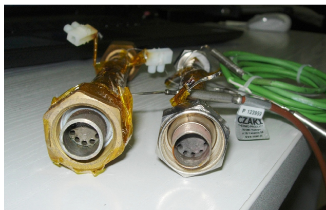
Fig. 2. Evaporator filled with a wick. Ni-Cu (left side) and Ni-Al (right side).
