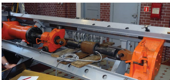
Fig. 7. Tests of the measurement module in the strength testing machine
