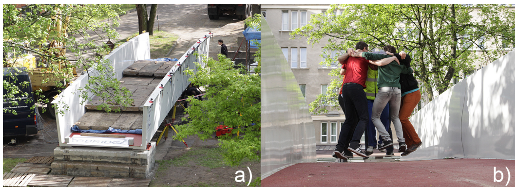
Fig. 12. Footbridge short-term testing: a) static load; b) dynamic load
