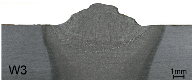
Fig. 3. Macro cross-section of the welded specimens W1, W2 i W3 (specimen without insulation W). Etch. Nital
