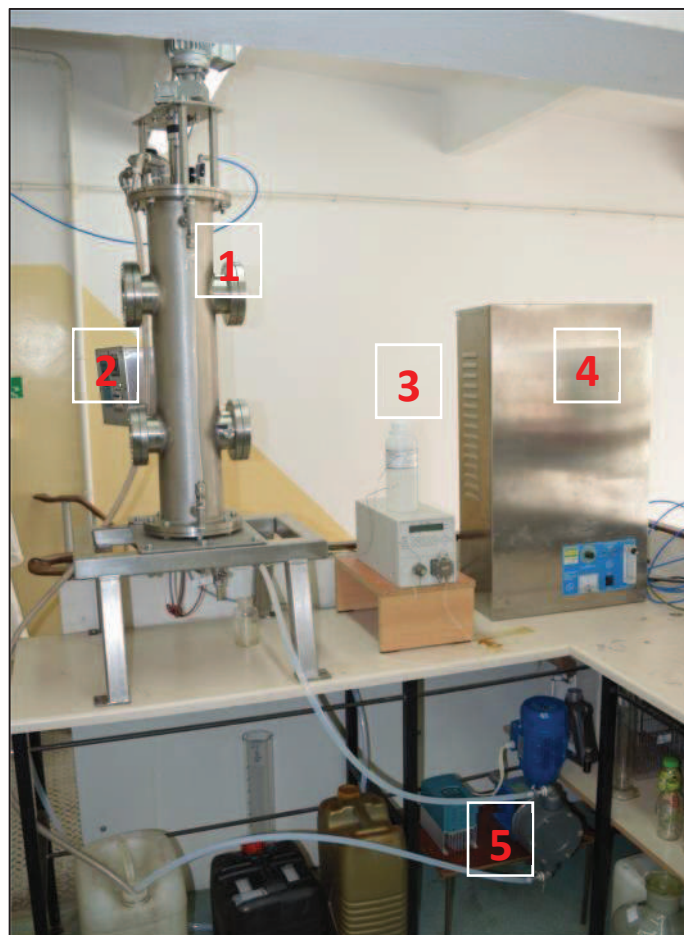
Fig. 1 A batch reactor for classic AOPs. 1- reactor, 2 – control panel (mixing and temperature), 3 – pump for oxidant, 4 – ozonator, 5 – pump for effluents
