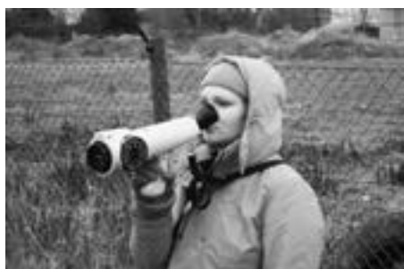
g. 3. D/T measurement using Nasal Ranger field olfactometers
