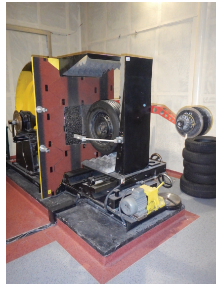
Fig. 4. Roadwheel facility with 1.7m diameter drum at the Technical University of Gdańsk, Poland
