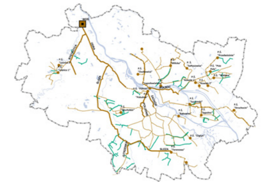
Figure 7 Sewage system: existing network
