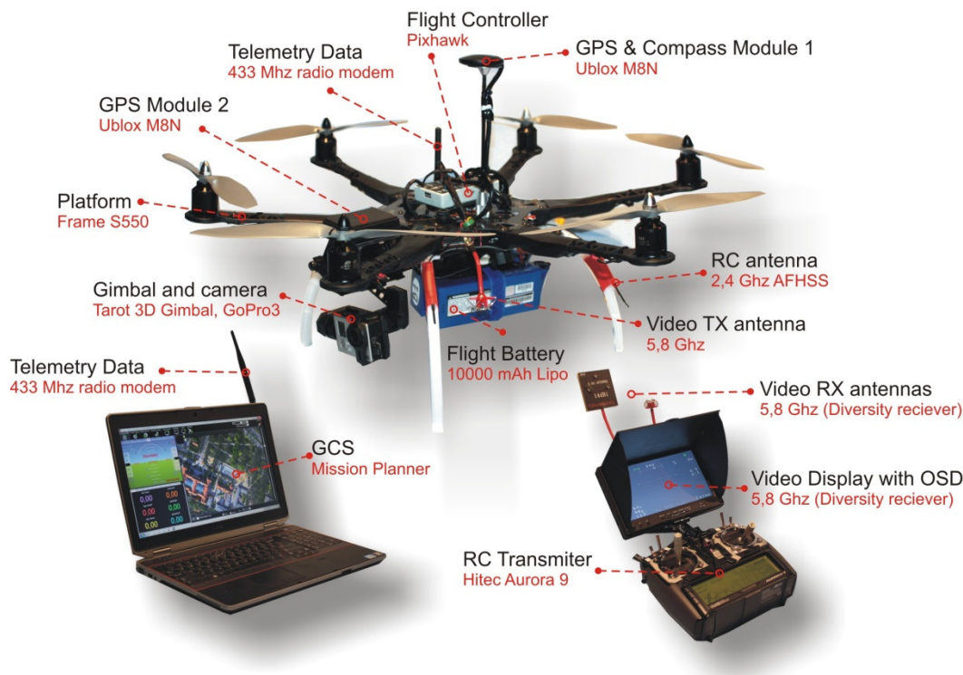
Fig. 2. Hexacopter platform hardware configuration and components assembly
