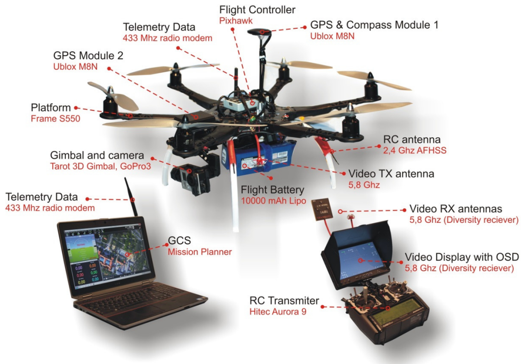
Fig. 2. Hexacopter platform hardware configuration and components assembly
