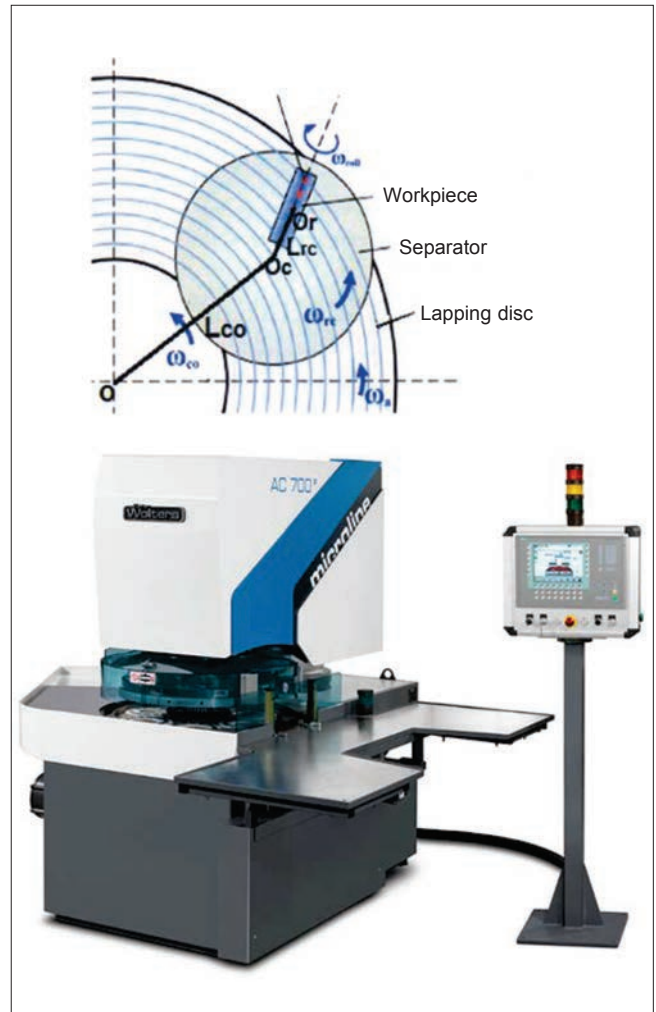
Fig. 6. Executive elements of the planetary system and the view of the Microline AC700 lathe by Peter Walters [8]
