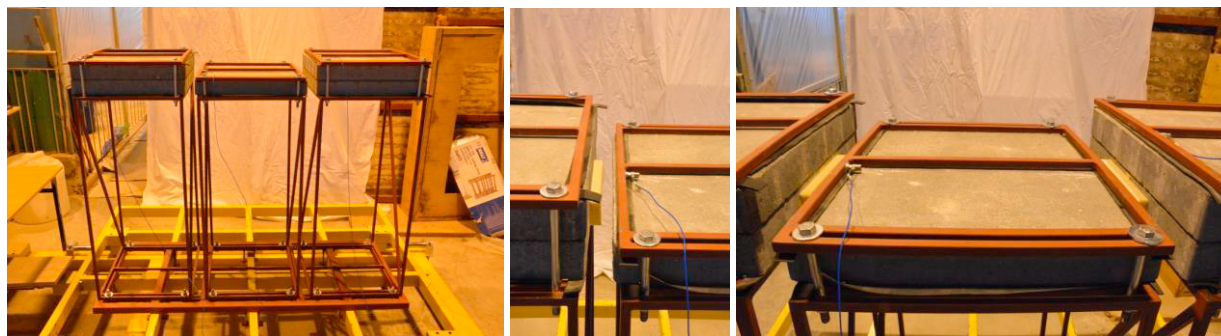
Fig. 1. Experimental setup and tower models with polymer elements with thickness of 20 mm.
