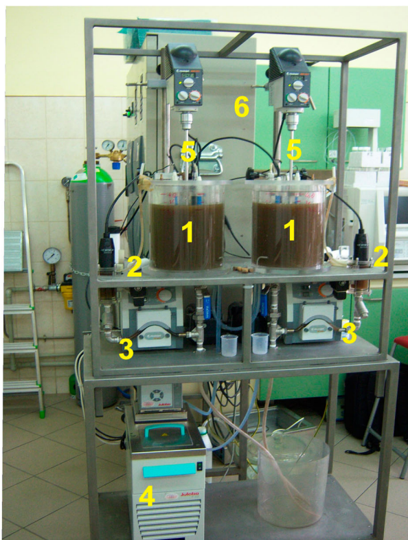
Photo 1. Experimental setup. 1 – batch reactors; 2 – units for the continuous measurement of oxygen uptake rate (OUR); 3 – peristaltic pumps; 4 – cooling/heating system; 5 – mechanical stirrers; 6 – control box; and 7 – computer control and data acquisition system.
