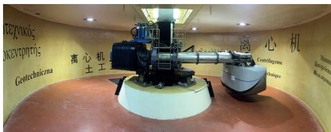
Fig. 1. Geotechnical centrifuge at Ifsttar [19].
