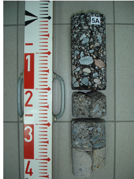
Figure 2. A specimen cored out at the crack in the national road No. 7. The crack propagates through the entire pavement.
