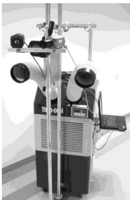
Figure 4. The ADT imaging unit used in the research
