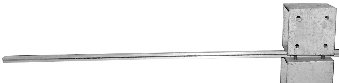
Fig. 1. A cantilevered aluminium beams with polymer adhesive inside.
