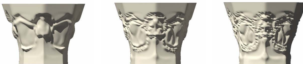
Figure 6. (a) Surface applied displacement generated based on the #1 ANN; (b) Displacement with sine function applied; (c) Displacement with 3*sine function applied;
