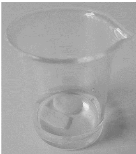
Fig. 3. Sample of bone cement immersed of SBF solution
