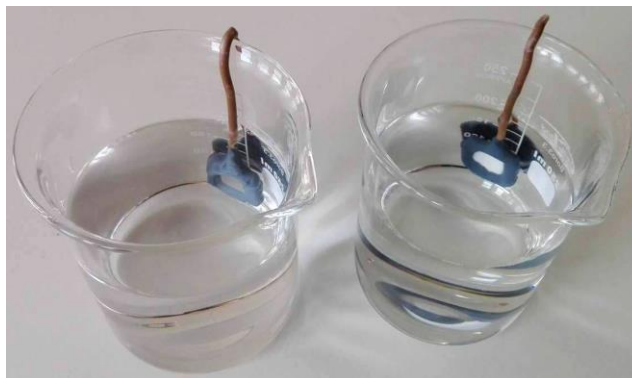
Fig. 1. Specimens immersed in artificial saliva
