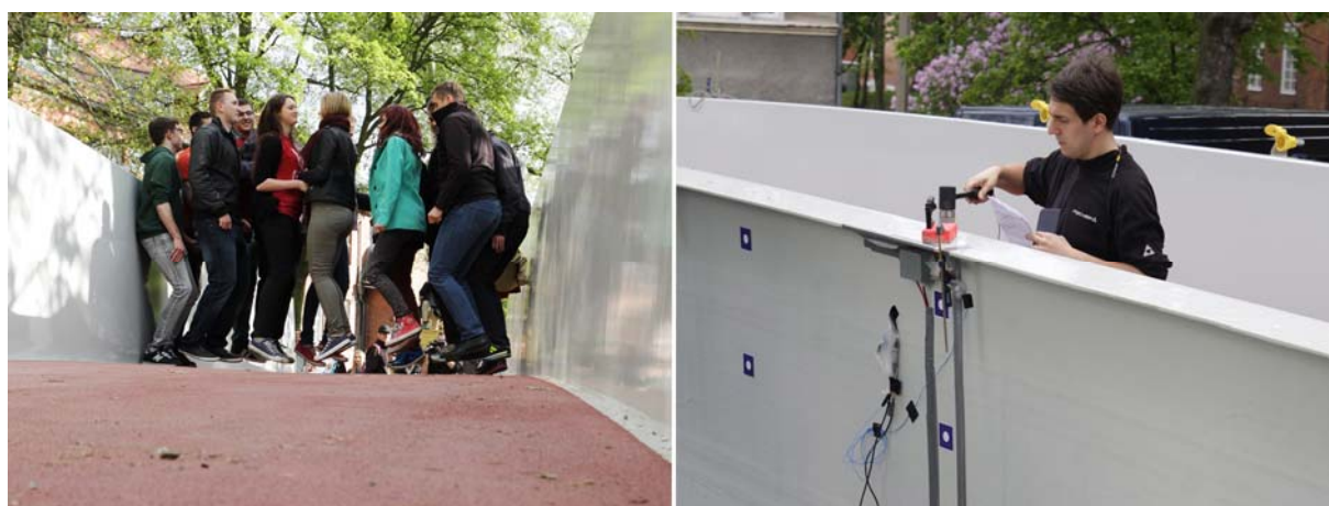
Figure 11. Dynamic loads: jumping (left), modal hammer (right)
