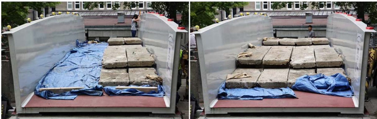
Figure 5. Footbridge loaded with ballast during static tests
