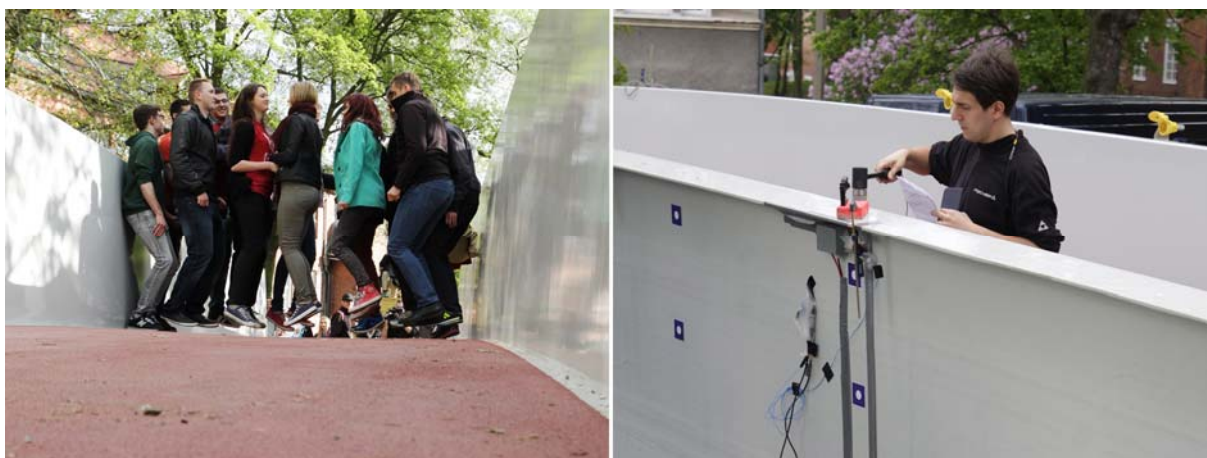
Figure 11. Dynamic loads: jumping (left), modal hammer (right)
