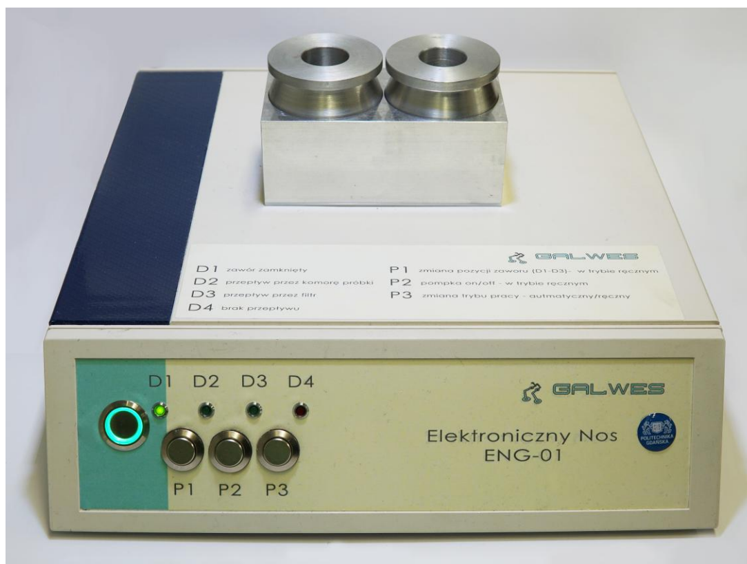
Figure 2. The view of an electronic nose prototype based on the electrochemical sensor array.
