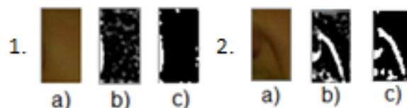
Fig. 5. Nose extraction in neutral (1) and contempt (2) emotions: (a) original image; (b) image after GL filter; (c) thresholded image.
