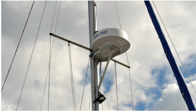
Fig. 4. Navigation device – radar
