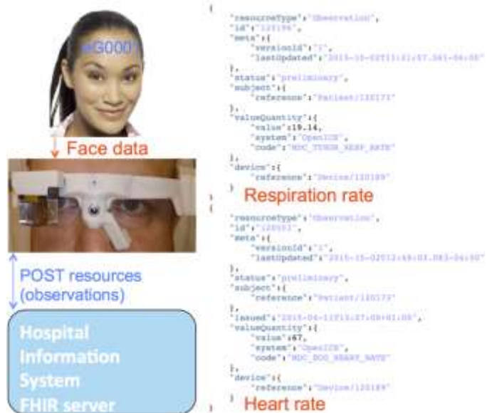
Figure 7: Estimated vital signs encoded using the HL7 FHIR standard for the exchange with healthcare information system.
