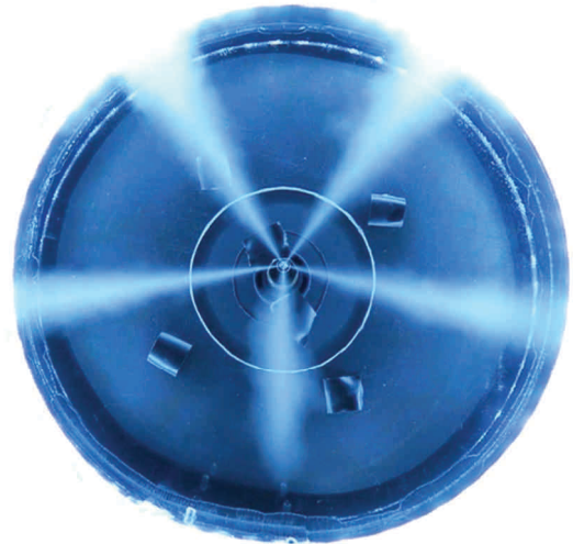
Fig. 20. Fuel spray pattern of a damaged injector
