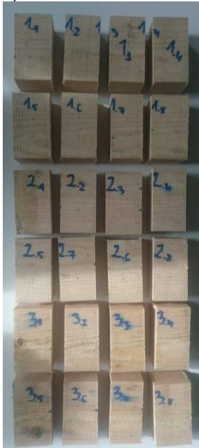
Fig. 4. The view of samples prepared for experiment: a) untreated, sawnwood, b) impregnated wood
