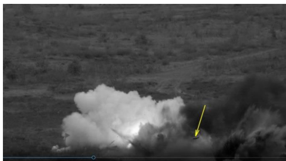
Fig. 15 Explosion of methane cylinder; the arrow indicates big shrapnel that moved over 500 m.
