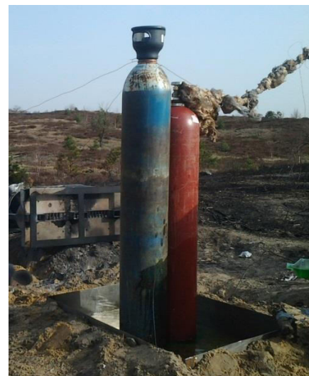
Fig. 22 Oxygen and acetylene cylinders before the experiment
