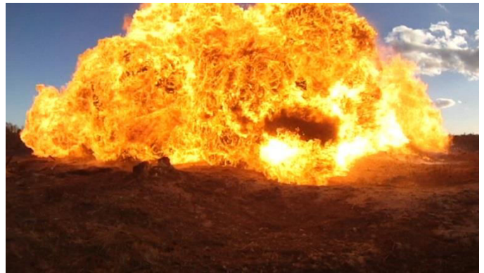
Fig. 21 Fireball developed after shooting through LPG cylinder
