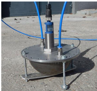
Fig. 2 Hydrogen sensor constructed at TUG
