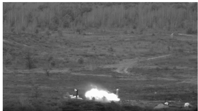
Fig. 14 Jet fire associated with shooting hydrogen cylinder.
