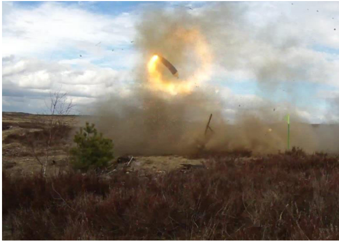
Fig. 11 Oxygen cylinder rotating after hit by bullet
