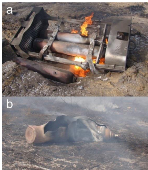
Fig. 9 Battery of cylinders after neutralization; a - the frame with one ruptured cylinder and two punctured cylinders, b - ruptured cylinder found 42 m away
