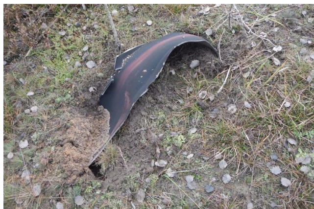
Fig. 24 Shrapnel created by blow of CO 2 cylinder
