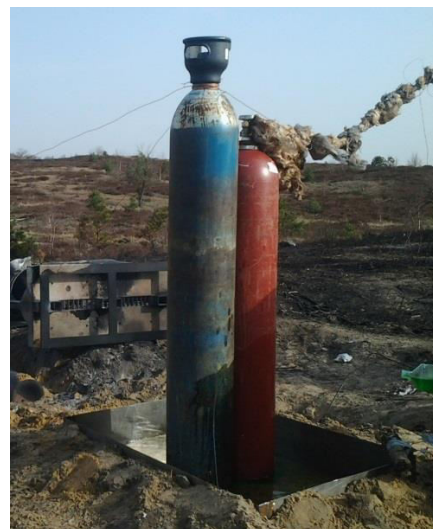
Fig. 22 Oxygen and acetylene cylinders before the experiment
