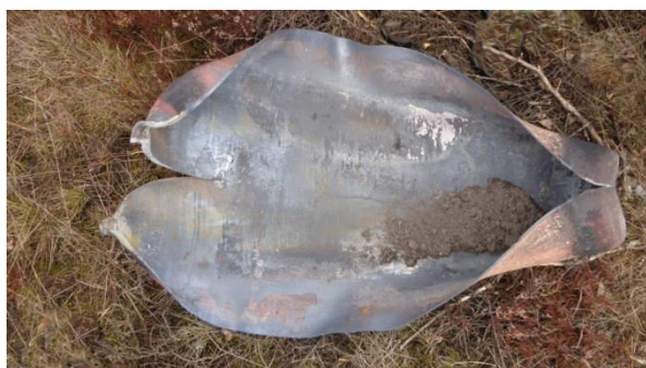
Fig. 5 Fully ruptured acetylene cylinder
