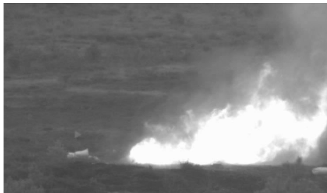
Fig. 17 Jet fire developed after hitting methane cylinder with bullet.
