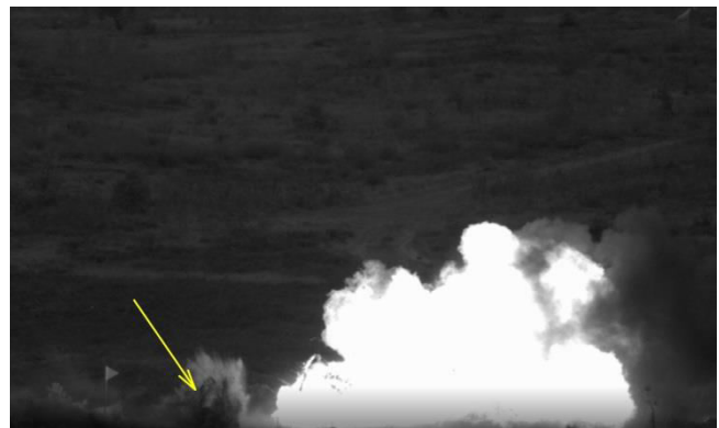
Fig. 13 Explosion of hydrogen cylinder; the arrow indicates place where big shrapnel buried into the ground.
