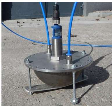
Fig. 2 Hydrogen sensor constructed at TUG
