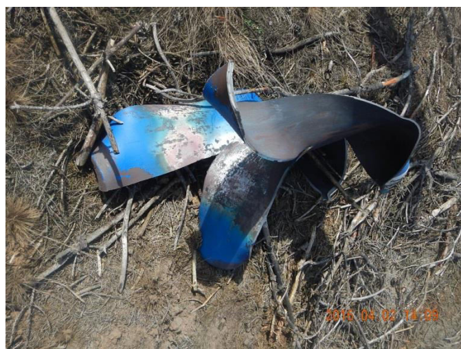
Fig. 10 Shrapnel created during the blast of oxygen cylinder that was thrown 146 m from the place of explosion
