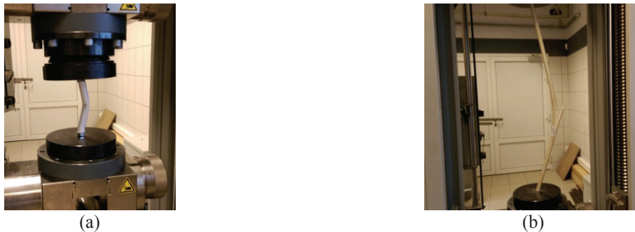
FIGURE 2. The test stand for compressive tests – a pinned support scheme for both PVC-U elements, where a bolt was used (a) and for timber elements, with a spherical ending formed by polishing (b) – photo taken after a buckling-induced plastic failure
