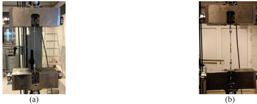
FIGURE 5. The test stand for tensile tests, where the tendons were installed in the clamps indirectly, through a snap hook – the nylon monofilament tendon is attached to the hook using a fisherman's bend knot (a) and the steel wire is clamp-gripped (b)
