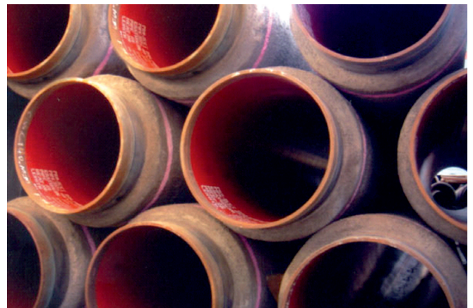
Fig. 1. Thick-walled steel pipe coated with 3M Scotchkote epoxy coating EP2306 HF, and a heavy concrete coating, for 370 km × 48 in. Dolphin (subsea) gas pipeline [10]
