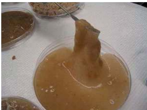
FIGURE 1. Biopolymer – sand viscous mixture (Knox and Petriso 2010)
