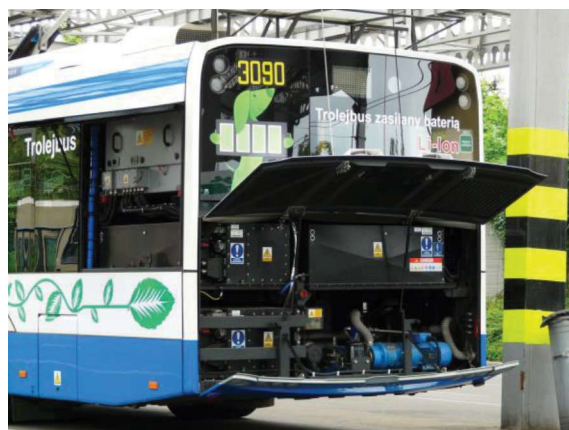
Fig. 5 Rear part of a Solaris Trollino 12 MEDCOM trolleybus, 3 battery modules (black boxes) and the charging system (a grey box in the upper part of the apparatus) are visible
