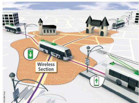
Fig. 1 The idea of In Motion Charging system (IMC) [© Vossloh Kiepe]
