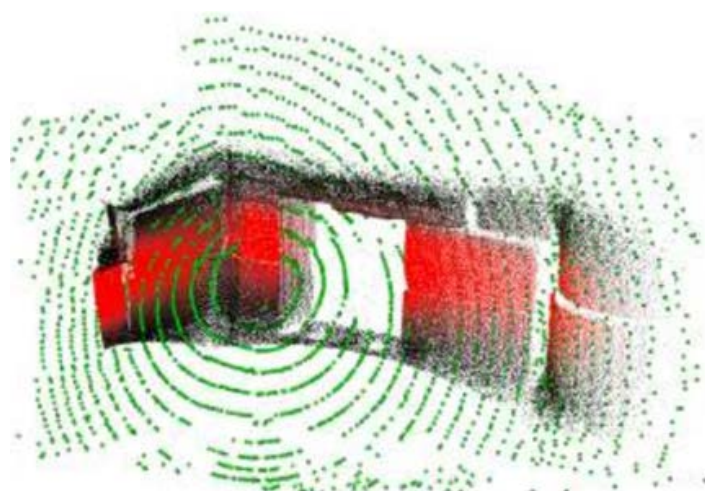
Fig.1. The differences in acoustic and laser measurements (green points - acoustic, black and red - laser) [6]
