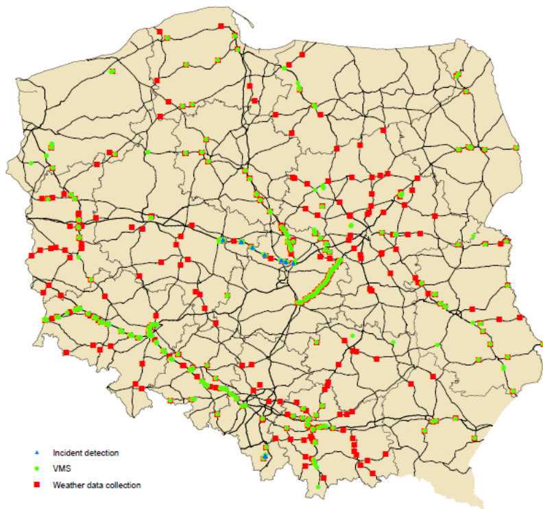
Fig. 1. Selected ITS devices on Polish national roads in 2015 [own study based on GDDKiA data]
