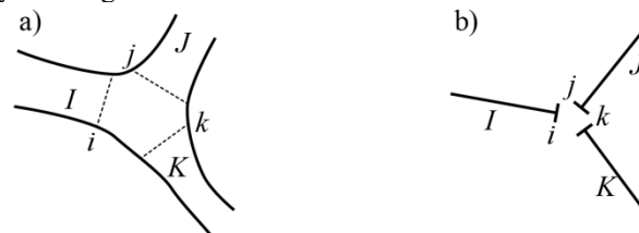
Fig. 9 (a) The sketch of the channel junction and (b) its typical computational representation.
