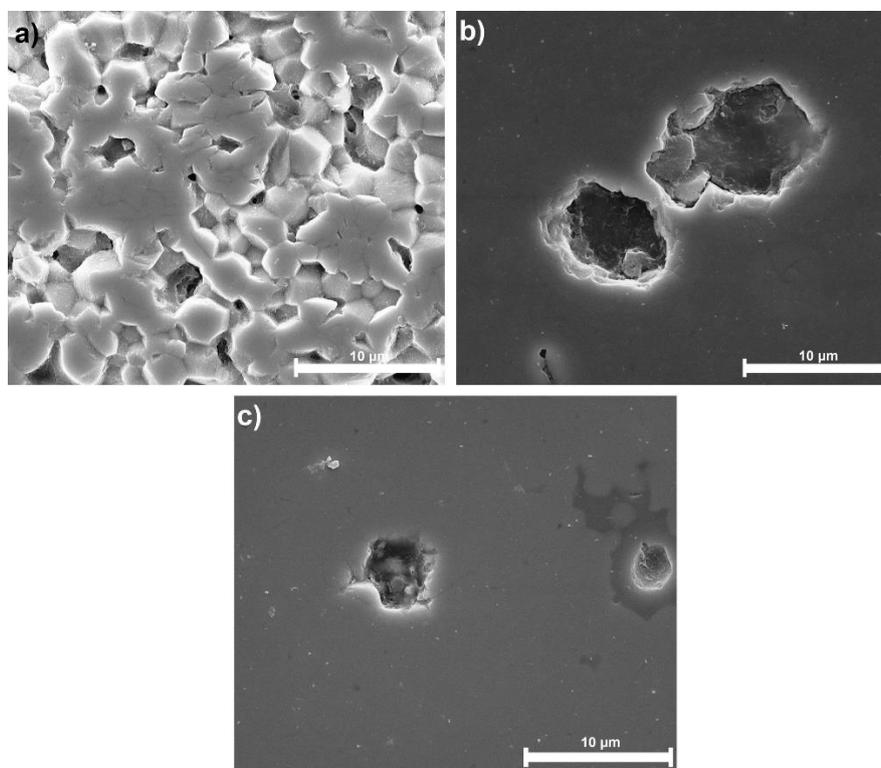
Fig.2. SEM photographs of a)  $\text{La}_{0.9}\text{Pr}_{0.1}\text{NbO}_4$ , b)  $\text{La}_{0.9}\text{Pr}_{0.08}\text{Ca}_{0.02}\text{NbO}_4$  and c)  $\text{La}_{0.88}\text{Pr}_{0.1}\text{Ca}_{0.02}\text{NbO}_4$ .
