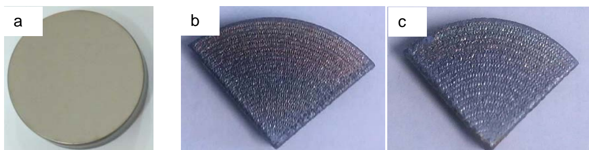
Fig. 1. Surface microstructure of the Ti13Nb13Zr alloy: a) before laser treatment and cut (BM) b) after laser treatment (LT 1), c) after laser treatment (LT 2)
