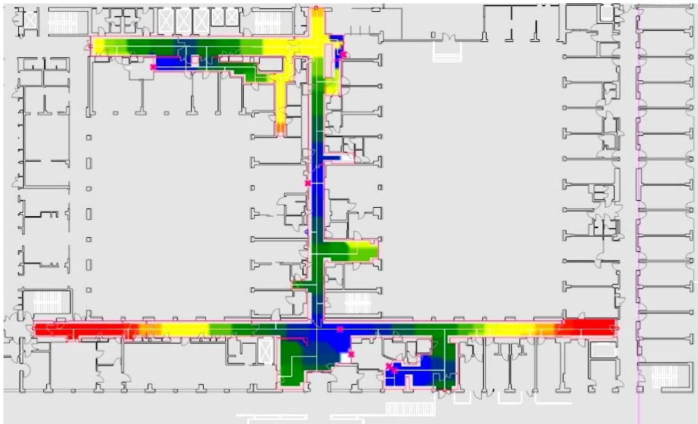
Figure 4. Visual representation of the access time analysis for nursing points. Emergency department of the Voivodship (Provincial) Hospital in Elbląg. A fragment of the 1st floor plan. Design: A. Kohnke, J. Bąkowski, 2014
