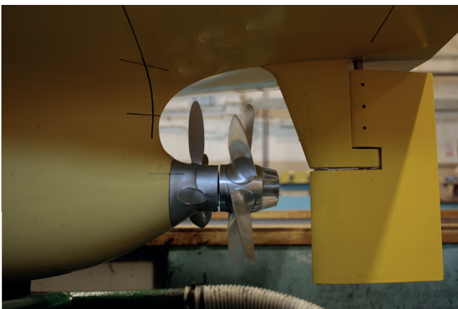
Fig. 6. Self-propulsion test arrangement with pre-swirl stator
