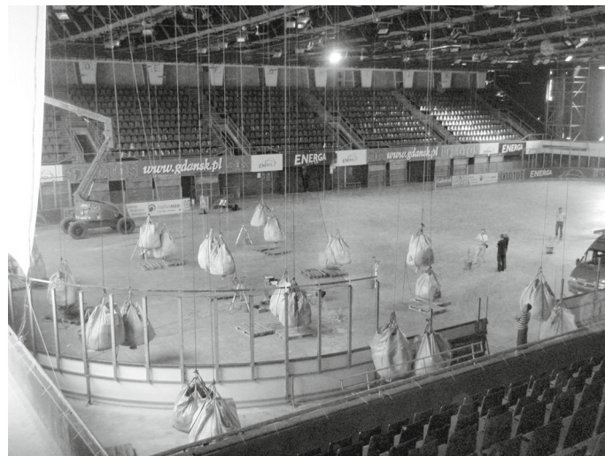
Fig. 18 Actual photograph of the static load due to hanging bags
