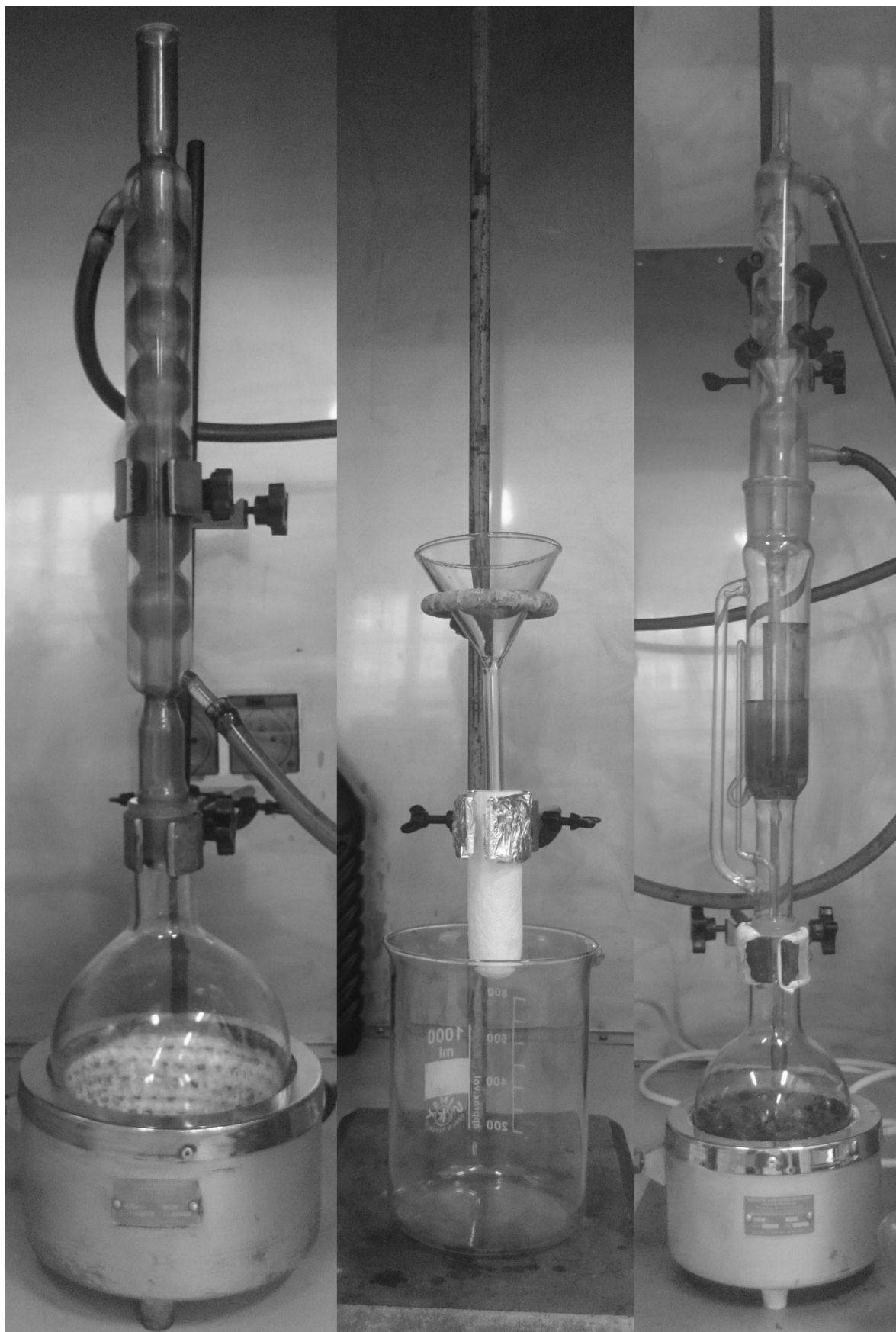
Figure 2. Experimental glassware setup. From left: precipitation set, filtration set, washing (Soxhlet) set. ( SINGLE COLUMN )
