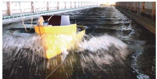
Fig. 1. The seakeeping tests in the CTO S.A. deepwater towing tank.
